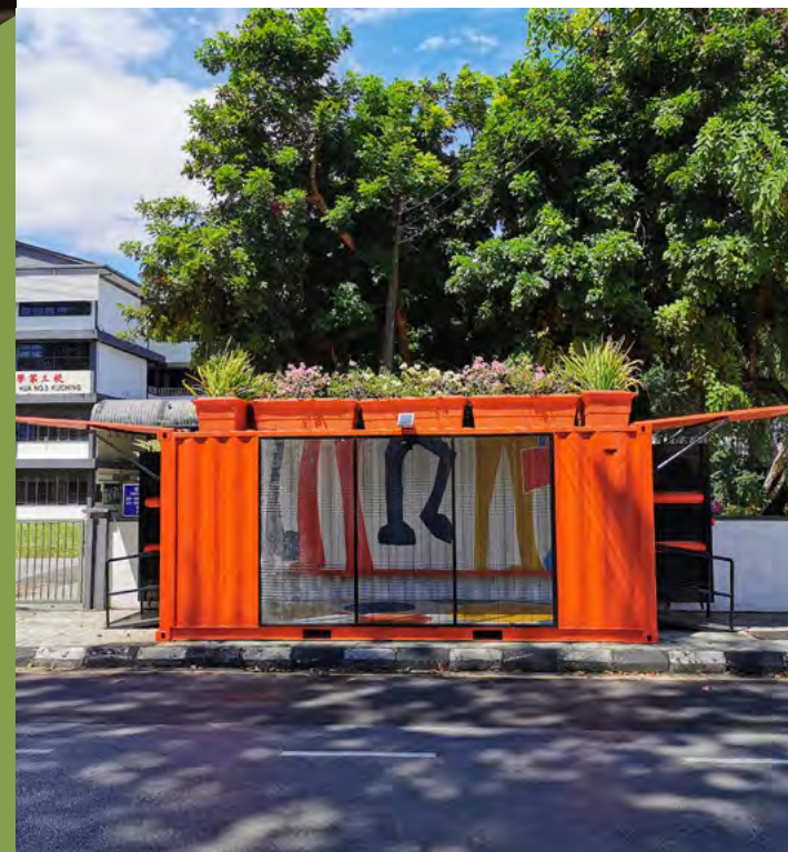
Planters placed on the roof by MBKS Landscape Department minimise heat gain from direct sunlight
