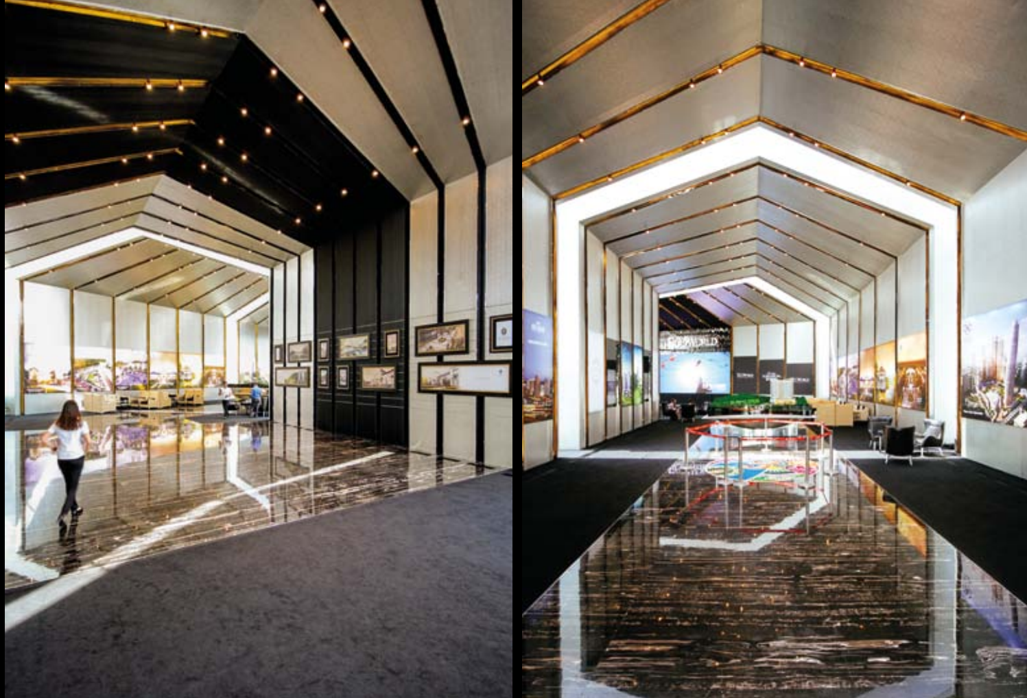
ABOVE: At the bend of the roof and walls, a continuous strip of skylight helps to bring natural light into the space
